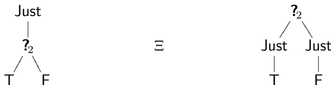
Figure 3.6: A simple example of pull-tab transformation (written \Xi ) to show the “unzipping” process that gives it its name. The Just node is duplicated (“unzipped”) to allow the choice to be moved toward the root of the expression.
